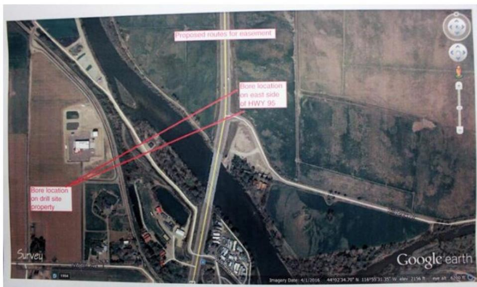
As currently planned by gas and oil producers, two lines that would be bored to a depth of 20 feet below the bed of the Payette River would pass close to the City of Fruitland's intake facilities for its drinking water plant.
