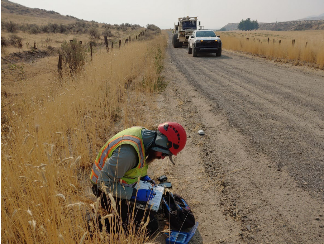
Seismic survey operations by Explor Geoscience Inc. along Big Willow Road, Payette County in August 2026.
