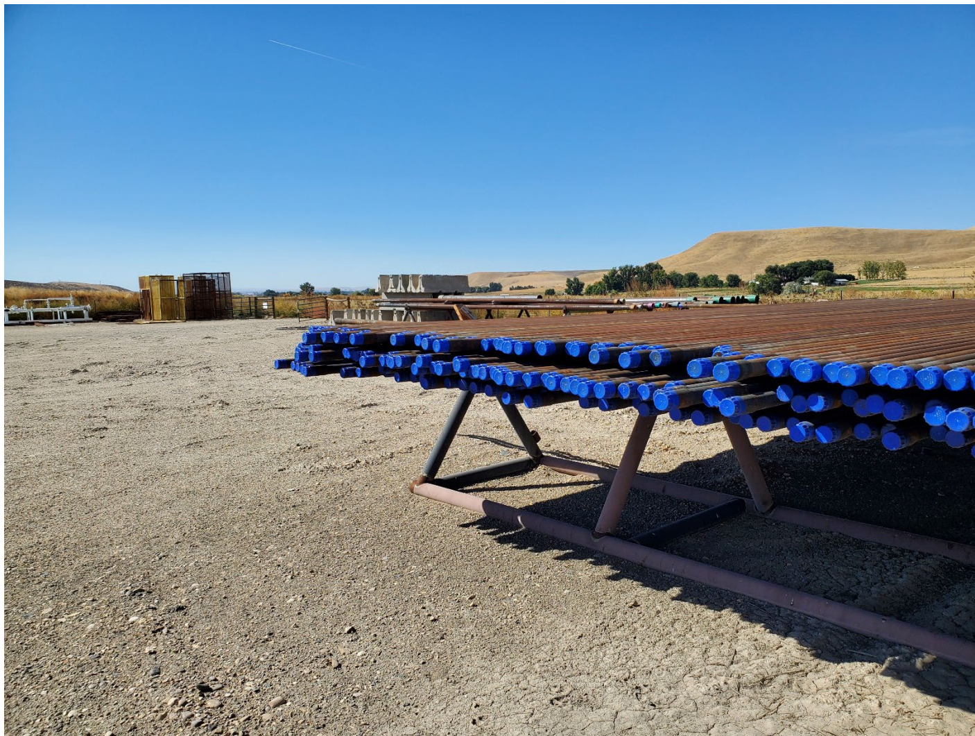
Tubing strings (foreground), casing sections and other equipment stored on site (background). View is Southwest.
