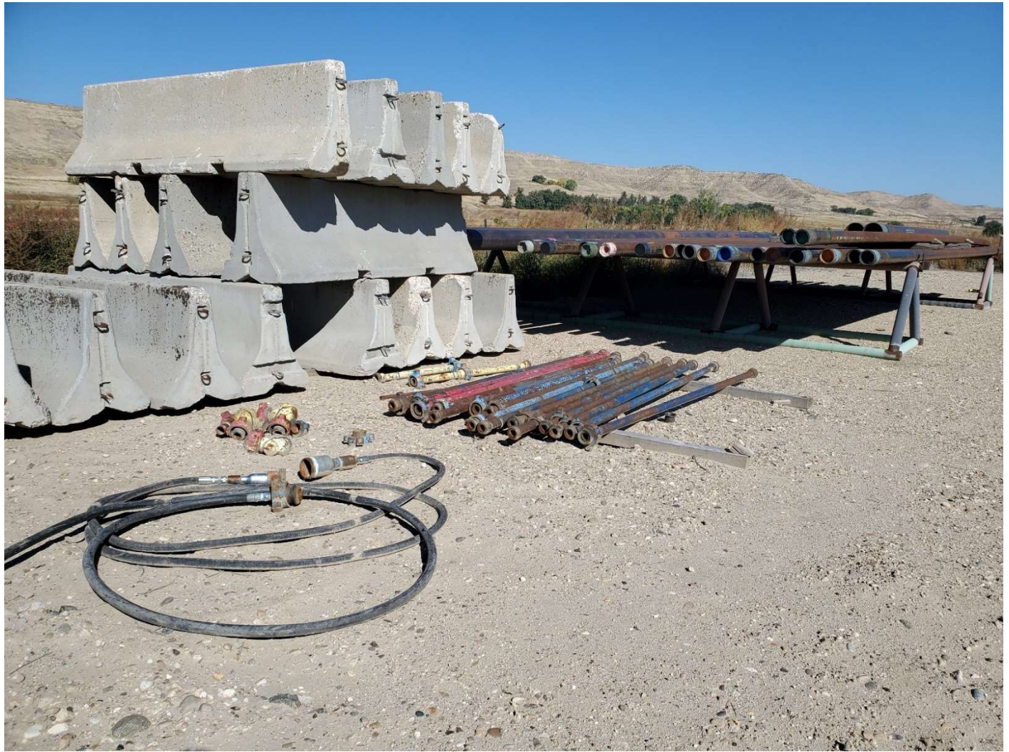
Casing, tubing and miscellaneous equipment stored on northwest perimeter of well pad. View is North.
