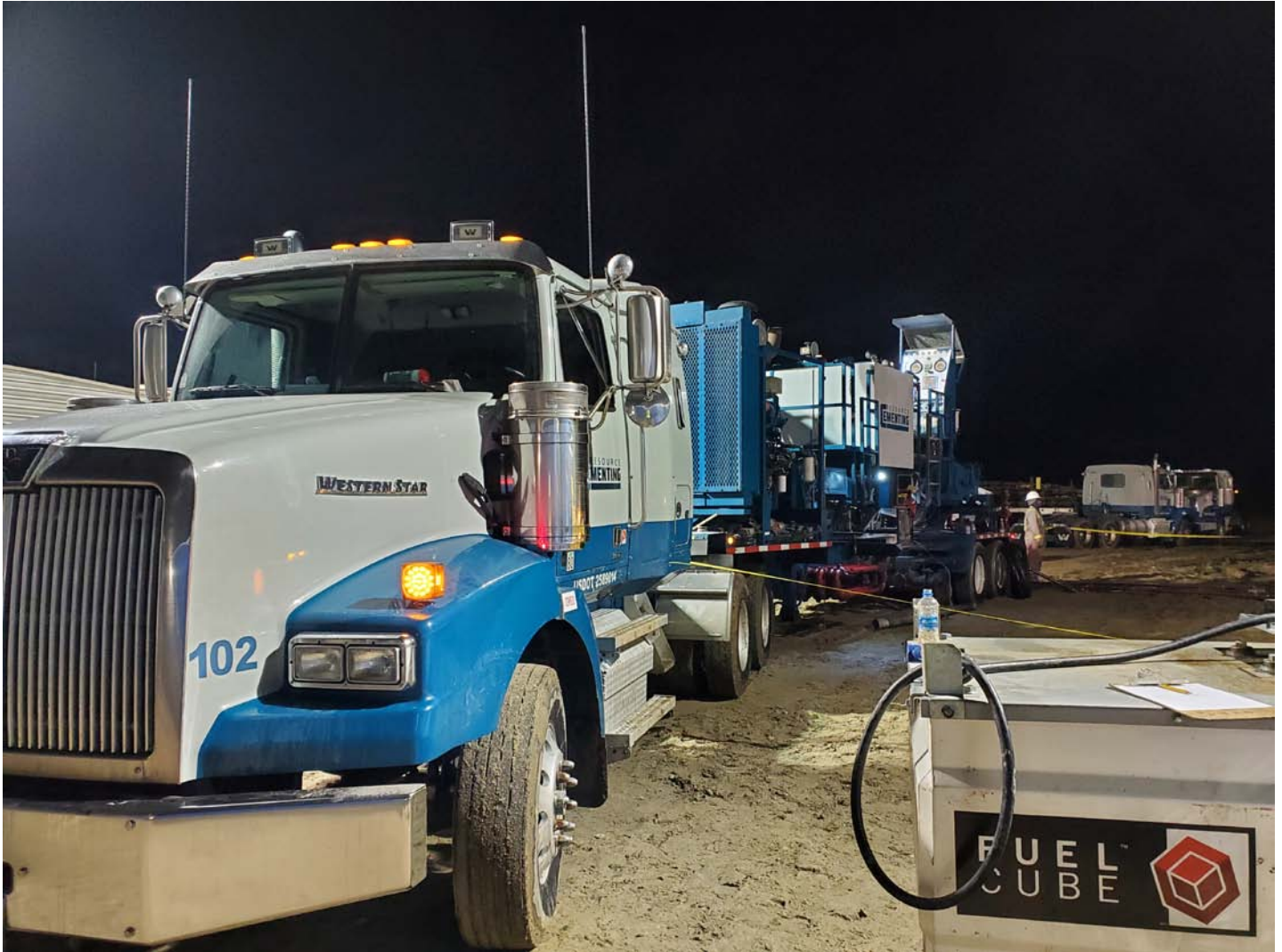
Resource Cementing equipment rig-up for surface casing cement job.
