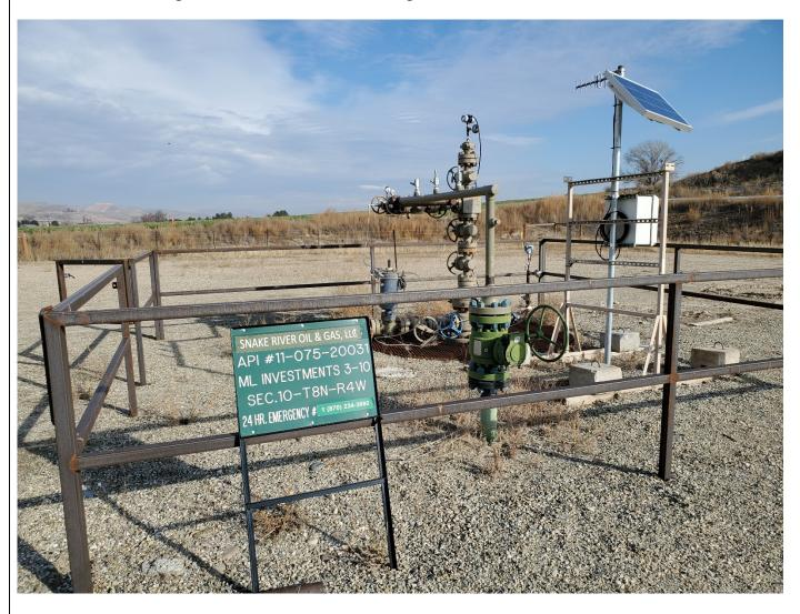
3. Wellhead showing analog and digital pressure gauges, grated cellar.
