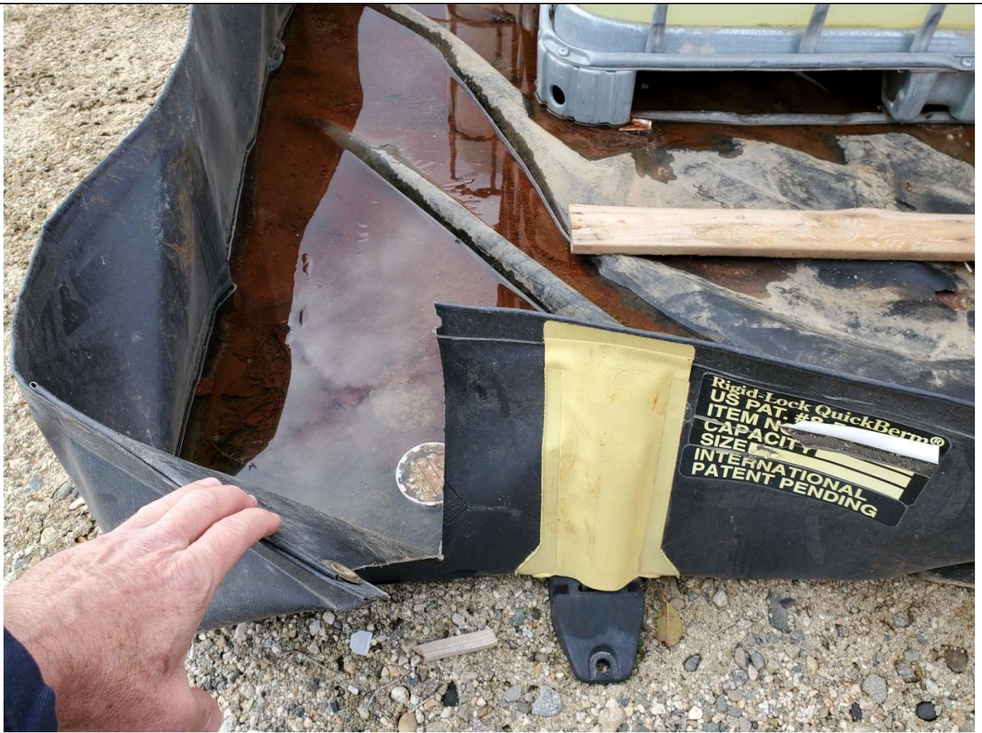
Detail of torn corner of auxiliary spill containment mat.
