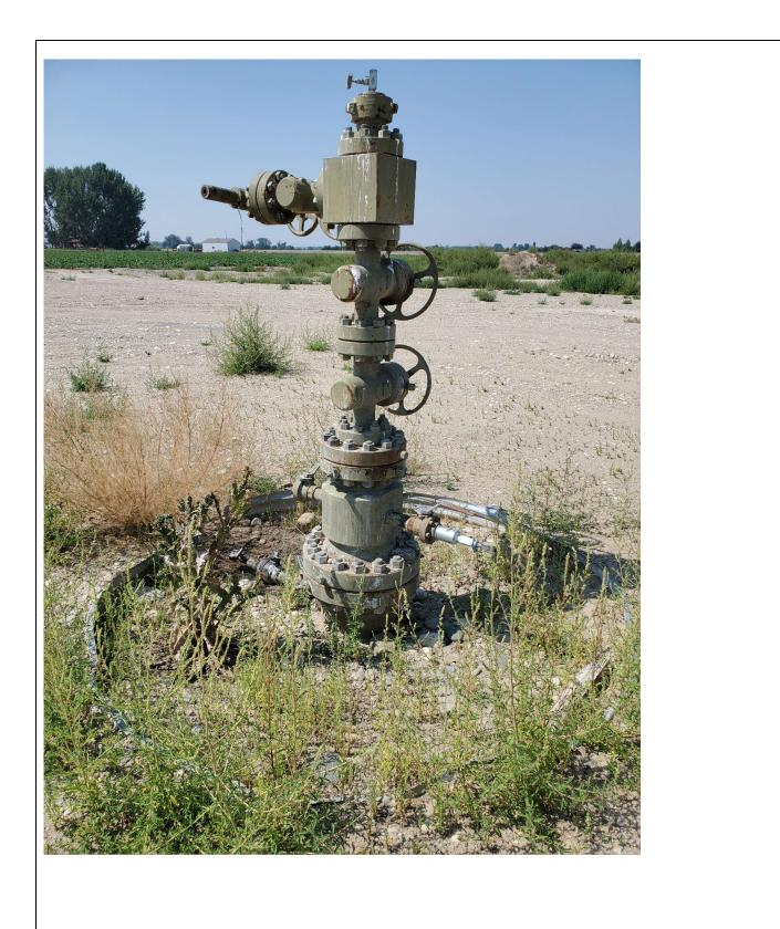
Photo 5: Tracy Trust 3-2 well head, 9 5/8" pressure gauge valve stem visible on lower right.
