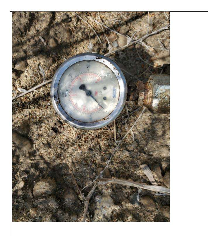
Photo 7: Tracy Trust 3-2 well head, 5 <sup>1</sup>/<sub>2</sub>" pressure gauge and valve stem visible on lower left. Valve is in the "Open" position.
